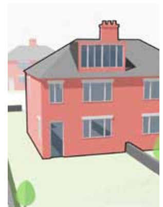
Image showing poorly-designed oversized dormer.
