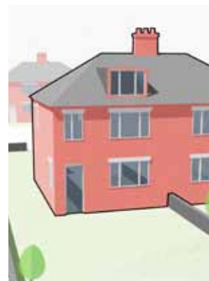
Image showing sensitive-sized and aligned dormer.
